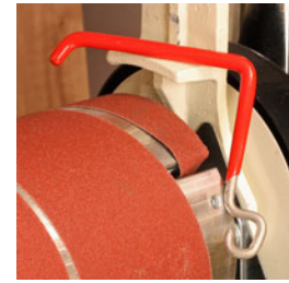
Our special Tuf Tool makes changing abrasive strips easier.
